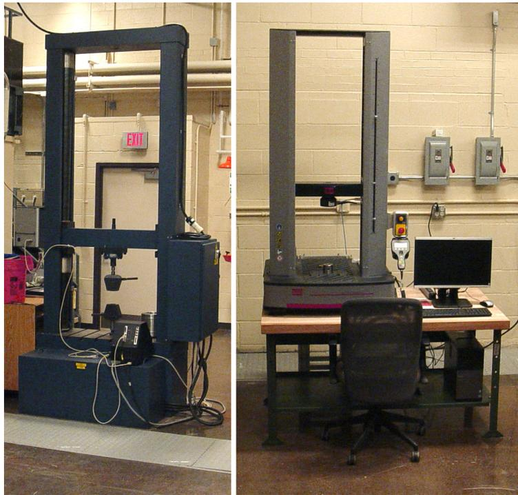
Mechanical test frames ranging from 6,750 to 100,000 lb load capacity
