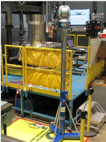
*Inspection Using Laser Tracker, Arm and Scanner*
