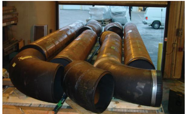
Prefabrication of feedwater piping for a piping replacement project
