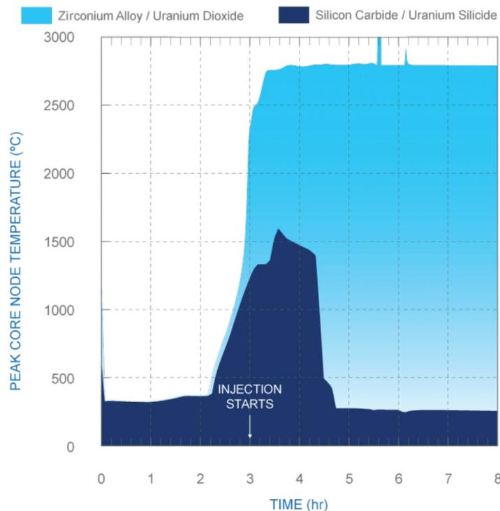
**Fig. 4.** MAAP modeling of a complete station blackout event with minimal cooling shows that silicon-carbide fuel will survive.
