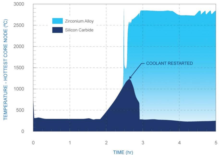
**Fig. 3.** Three Mile Island-2 progress simulation: Silicon-carbide cladding tolerance to heat and steam as compared to that of TMI-2's zirconium alloy cladding.
