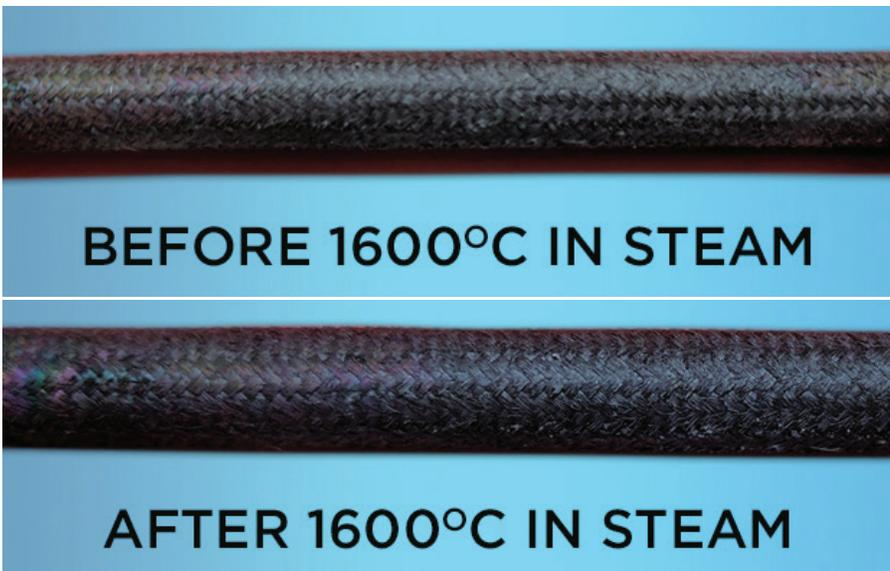
**Fig. 2.** Before and after photos of silicon-carbide cladding severe accident testing at about 1600 °C (about 2900 °F) for 40 minutes in steam. The cladding exhibited essentially no change or damage.
