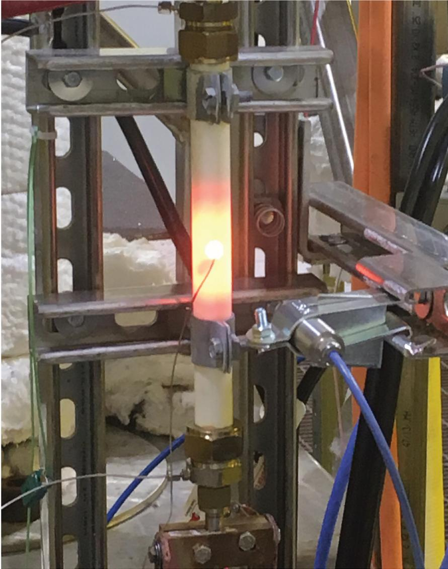
**Fig. 1.** A simulation of a severe accident test of silicon-carbide cladding at about 1600 °C (about 2900 °F) is carried out at Westinghouse's Ultra-high Temperature Test Facility. (Photos and graphs: Westinghouse Electric Company LLC)
