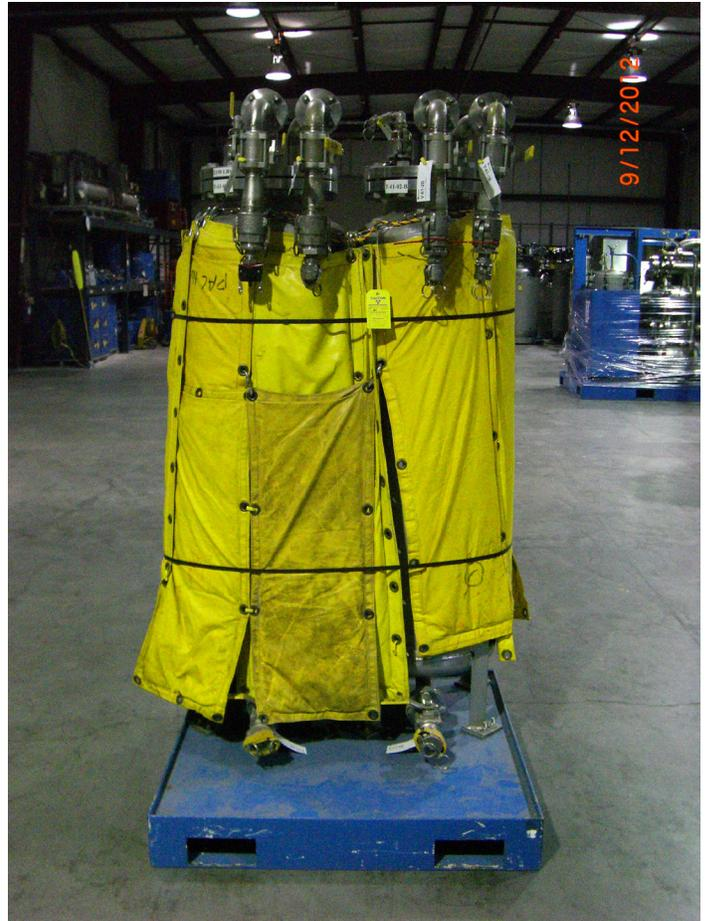
Shielded ion exchange columns on skid
