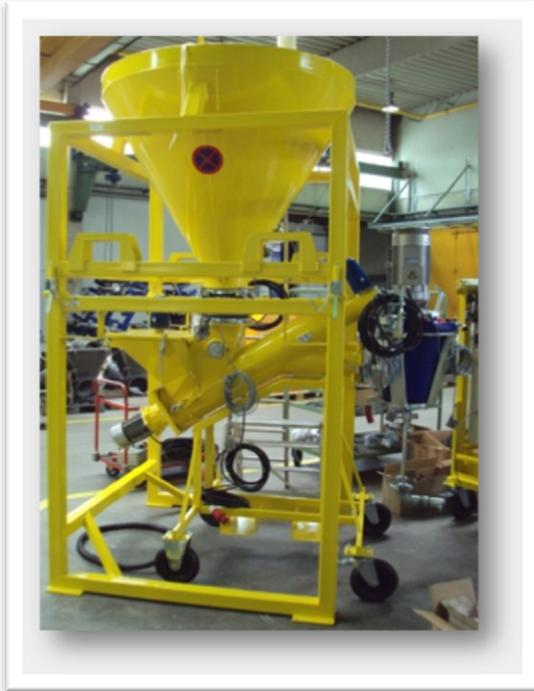
*Westinghouse grouting system with interchangeable silo*
